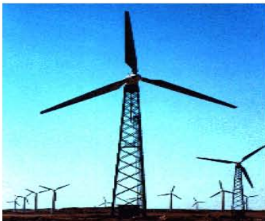
Nordtank Danish WT, Stall regulated, Lattice tower, 300 KW
